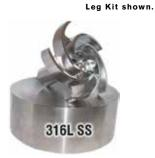
All Wet-end components are made from wrought 316SS, (UNS 31603) bar or flat stock with composition and manufacturing process controls that limit delta ferrite content to less than 5%.
